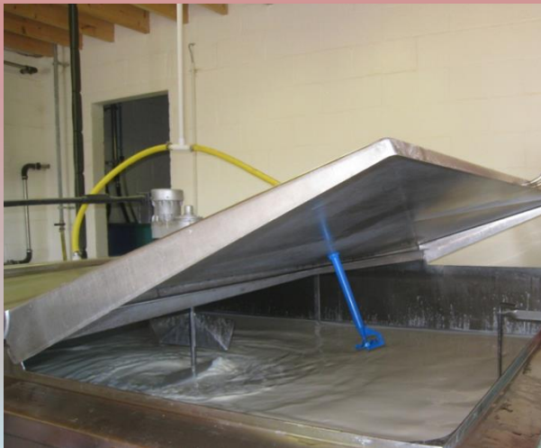
Dr. Omar Hashim Sheet Fig. 1. Bulk cooling tank with agitator and chilling unit
